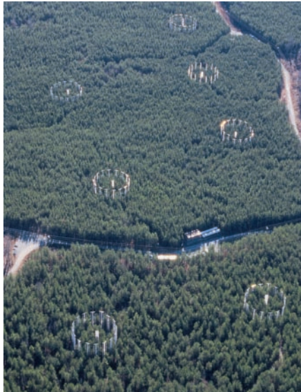
Fig. 1. Free-air CO 2 enrichment (FACE) rings in a pine plantation in North Carolina, USA. Each ring is 30 m in diameter and circumscribes about 100 trees. The distance from the single ring in the southwest (top right) to the two rings in the north (bottom) is ~500 m. The single ring in the background is a prototype. There are six experimental rings; three rings receive ambient air and three receive ambient plus 200 μl liter -1 CO 2 (photo: Will Owens).
