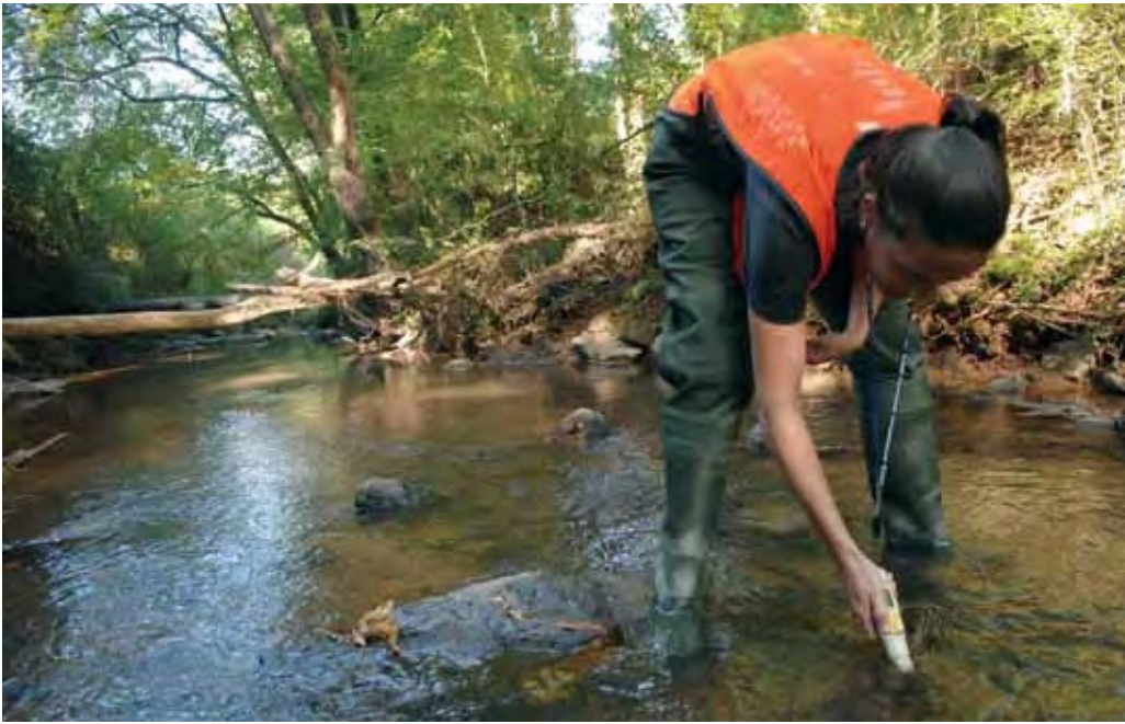
Environmental Practicum law student Becky Gabelman uses a probe to test water temperature and bacterial levels of Calls Creek in Watkinsville. The practicum is assisting the community in identifying and eliminating sources of fecal coliform to the stream.
